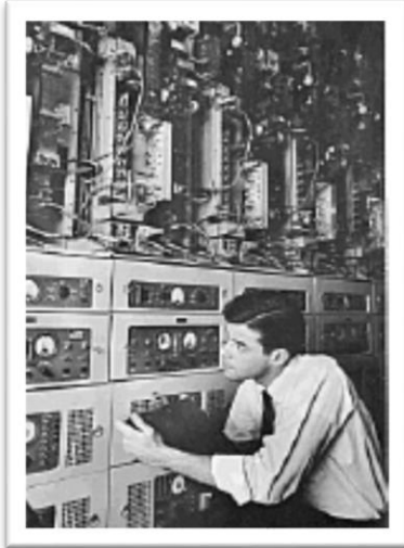
San Francisco-New York transcontinental route of 4 GHz TD2 analog FM-FDM hops completed in 1951 for long distance VF and TV
